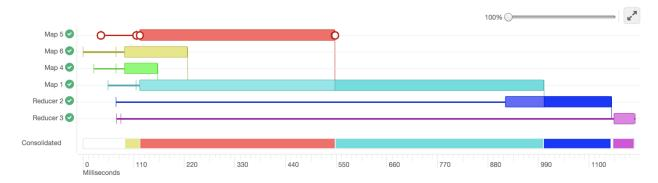
Each horizontal bar of the swimlane represents the total time taken by the vertex to complete. The vertical lines indicate the time when the vertex initialized, the time when the vertex started, the time when the first task started, the time when the last task completed, and the time when the vertex finished its execution. When you mouseover the vertical line, the bubble displays the stage of the vertex execution and provides a timestamp.
