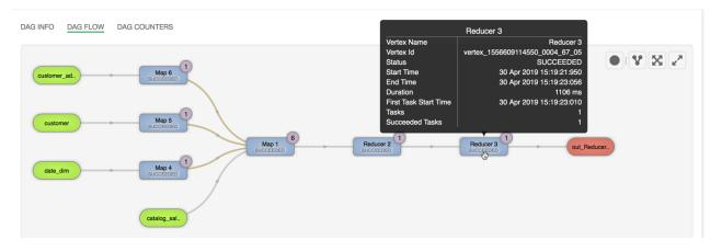
Here, the inputs to vertices Map 4, Map 5, Map 6, and Map 1 are the tables displayed in green boxes. Next, Map 1 depends on the result set generated by Map 4, Map 5, and Map 6. Map 1 then passes its result as an input to Reducer 2. When the Reducer 2 finishes its execution, the results are passed on to Reducer 3. Reducer 3 is the last vertex in the DAG flow. After the Reducer 3 successfully completes its execution, the query output is written to a file in HDFS.
